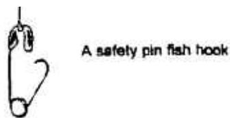
The fishing line can be used with a safety pin fashioned into a hook for fishing
